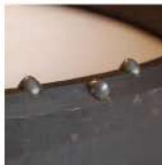
Press-fit ballistic carbide insert – flush O.D. shoe
